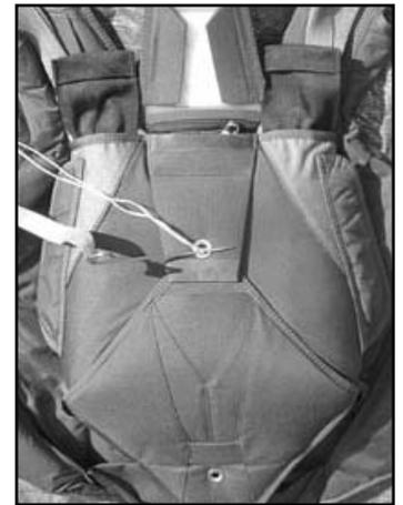
Feed the reserve cable through its housing until the pin appears out of the housing. Secure reserve handle between scratches. In case of a RSL use, please report to the Advance "Out" guide for setting instructions. Replace temporary closing pin with the reserve closing pin. Removed pull up cord and count your tools. Seal reserve pin with 5lg seal thread if mandatory in your country.
