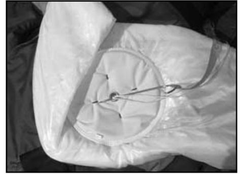
Thread the pull up cord through the #3 right closing flap. Remove and replace temporary pin.
