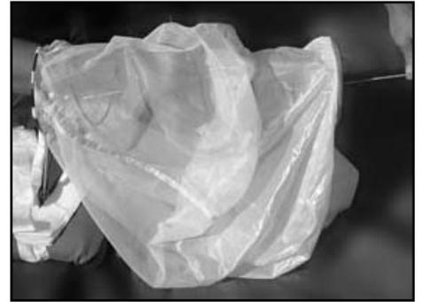
Center the pilot chute base over the #1 closing flap grommet.
