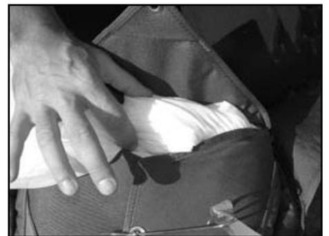
Thread the pull up cord through the #5 lower closing flap. Remove and replace temporary pin.
