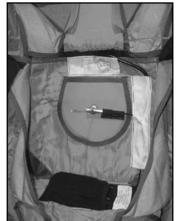
Install the A.A.D. main unit in its pocket, cable connexion must be facing downward. Airtec installation kit is only allowed for Cypres A.A.D. type. Stow remaining cables and route the cutter toward the lower reserve flap through the smallest channel. Control unit must be route in the white type 4 /1.5" channel toward the collar.
