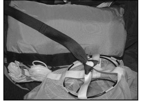
Main bag must be set into the main container, lines toward the bottom part of the container. Connecting bridle is folded up and down over the main bag. Main spring pilot chute is set over the bag and compressed by leaving netting into the spring.
