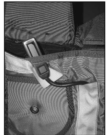
Slip the control unit in the back-pad and stowed it in its place. Reset the protecting flap. Installation is finished. It is possible to set the control unit in the right ring cover (only available for student Cypres unit on request).
