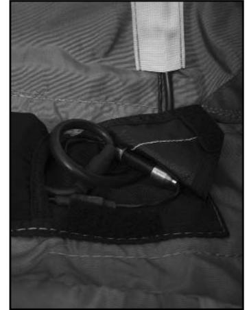
Close the protecting scratch flap. Set the cutter in its elastic band. Route the control unit through the slit at collar level.
