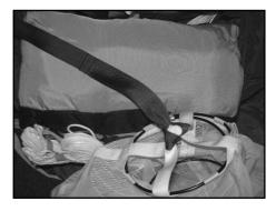
Main bag must be set into the main container, lines toward the bottom part of the container. Connecting bridle is folded up and down over the main bag. Main spring pilot chute is set over the bag and compressed by leaving netting into the spring.
