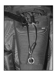
Install the A.A.D. main unit into its pocket, cable connexion must be facing downward. Airtec installation kit is only allowed for Cypres A.A.D. type. Stow remaining cables and route the cutter and the control unit in the white type 4/1.5" channel toward the collar.
