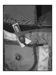
Slip the control unit in the back-pad and stowed it in its place. Reset the protecting flap. Installation is finished. It is possible to set the control unit in the right ring cover (only available for student Cypres unit on request).
