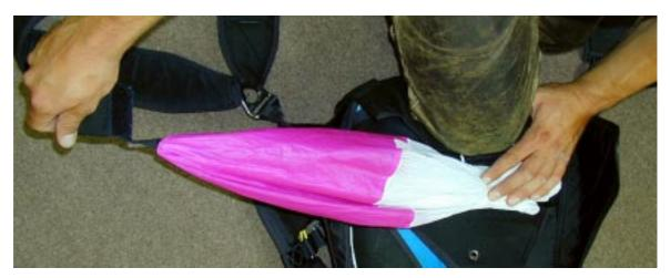
Hold the pad with your right hand and place the pilotchute in a way, so that the end of the mesh is in line with the left side of the main container. Place the pilot chute right on top of the loop keeper
