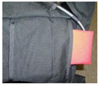
The AFF 2nd release ( shown from the side ). The pad is located under a velcro cover. To the left you'll find the pocket for the static line hook.
