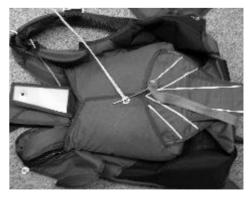
**# 17** Thread the pull-up cord through the reserve top flap #6 and insert the TLP you used on flap #5.
