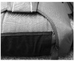
**#9** Make sure that your main risers are exactly placed on top of the lower closing flap of the reserve container.
