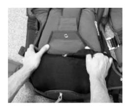
**# 4** Thread a pull-up cord through the closing loop on the bottom flap and thread the pull-up cord through the grommet on the #2 top flap.
