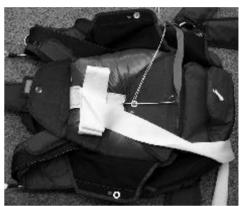
**# 11** Now close top flap #2 and secure it with the temporary locking pin (TLP) you used on bottom kicker flap #1.
