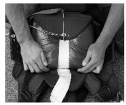
**# 10** S-fold one third of the bridle (5-6 small folds) on top of the free-bag (underneath top flap #2).
